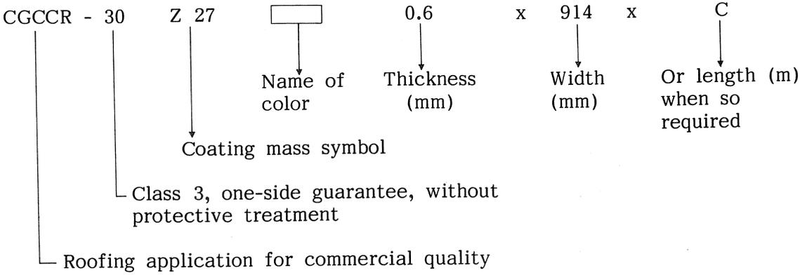
Figure 4 c) — For roofing (coil)
