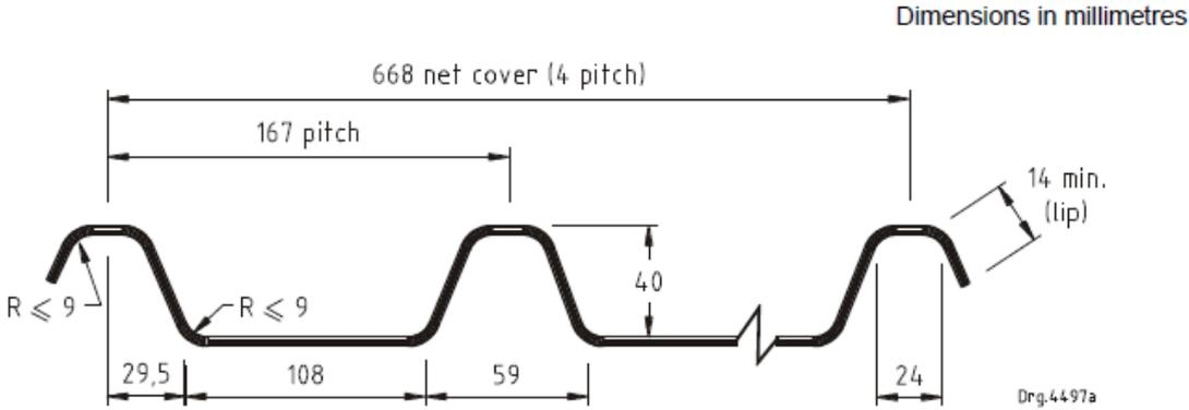
Figure 4 — Profile for troughed sheet — Type C
