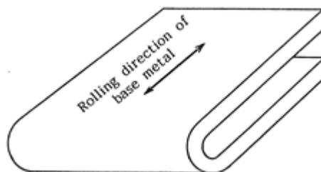
Figure 1— Direction of bend test
