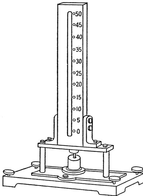
**Figure 3 — Du Point Impact-deformation tester**
