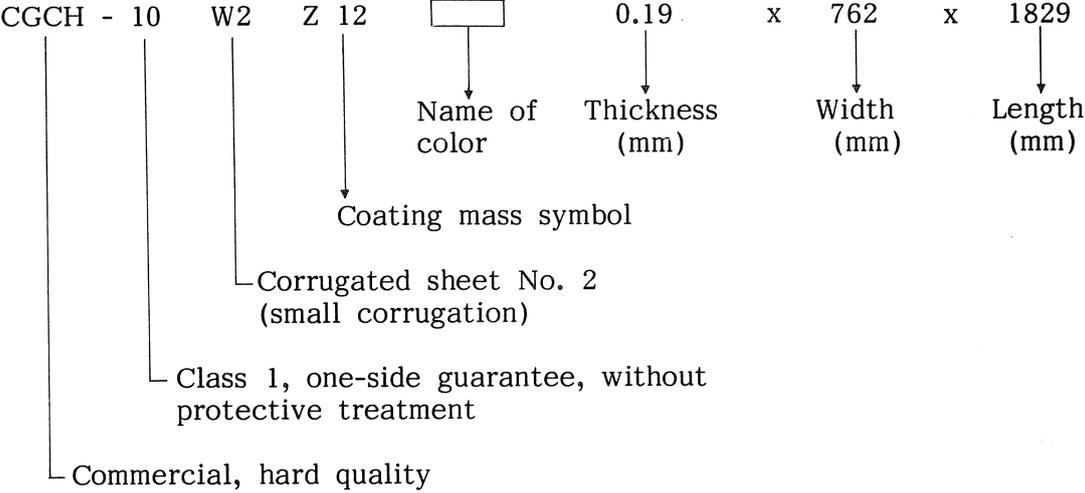
Figure 4 d) — For corrugated sheet using commercial, hard
