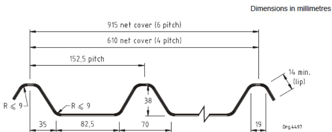
**Figure 3 — Profile for troughed sheet — Type B**
