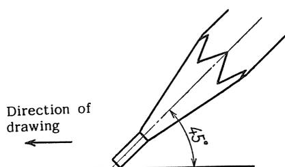
Figure 2 — Pencil hardness testing method
