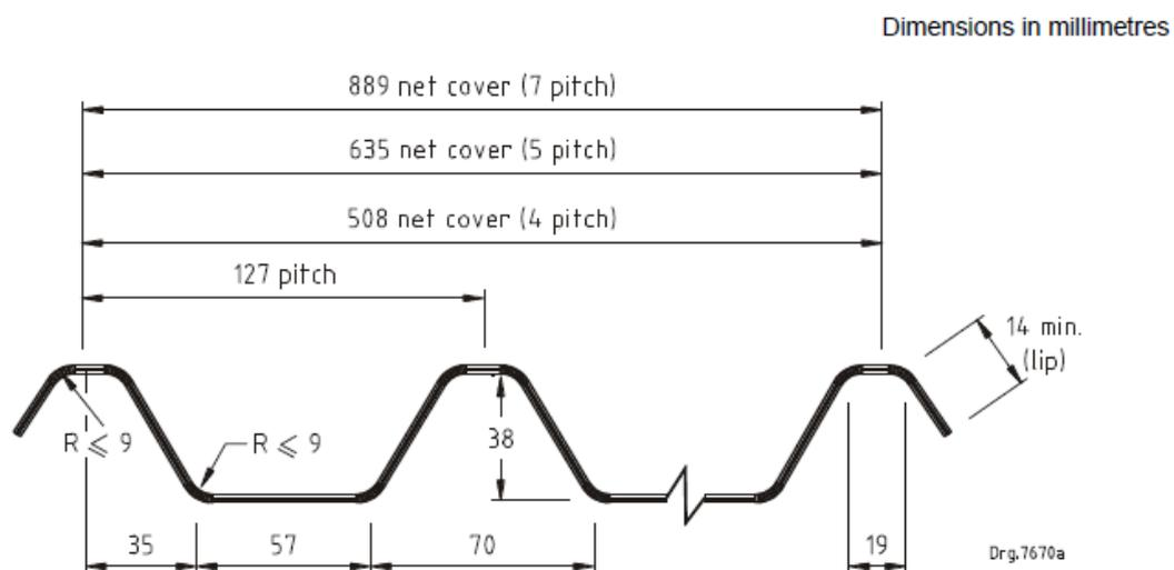
**Figure 2 — Profile for troughed sheet — Type A**
